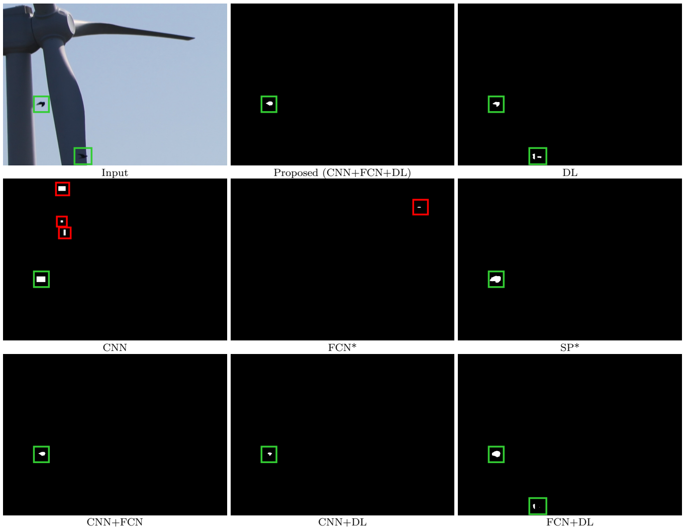
Fig. 4 Examples of typically misdected regions. The red squares mean false positives. CNNs are prone to the regions around the hub. FCNs are prone to the tips of the blade.
