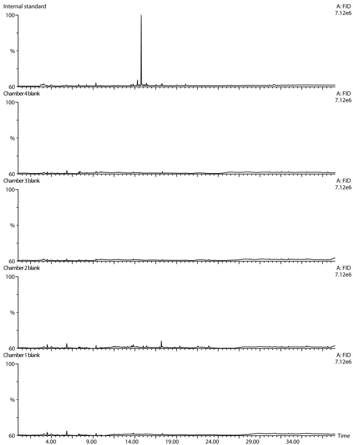
**Fig. S2.** FID chromatograms of internal standard and empty measurement chambers
