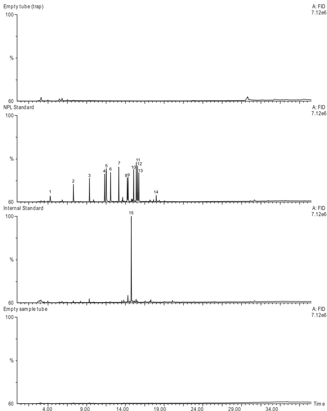
**Fig. S1.** FID chromatograms of an empty tube (trap); NPL gas standard with following compounds: (1) isoprene, (2) benzene, (3) toluene, (4) ethylbenzene, (5) m- and p-xylene, (6) o-xylene, (7)  $\alpha$ -pinene, (8) myrcene, (9)  $\beta$ -pinene, (10)  $\Delta^3$ -carene, (11) p-cymene, (12) limonene, (13) 1,8-cineole and cis-ocimene, (14) camphor; internal standard with (15)  $\Delta^2$ -carene and empty sample tube.
