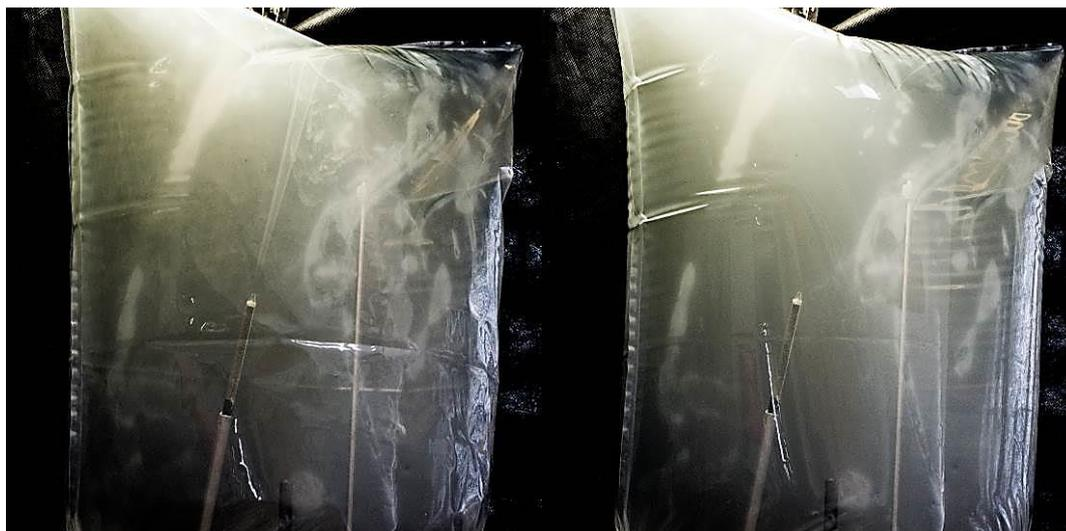
**Fig. S3 Gas mixing test.** Turbulent mixing within the chambers (left: no flow, right:  $10 \text{ l}_n \text{ min}^{-1}$ ). Black background and upward light installed to improve visibility (see video is available in Additional file 2). White areas in the left chamber represent the highly concentrated sulfuric acid particles leaving the smoke tube.
