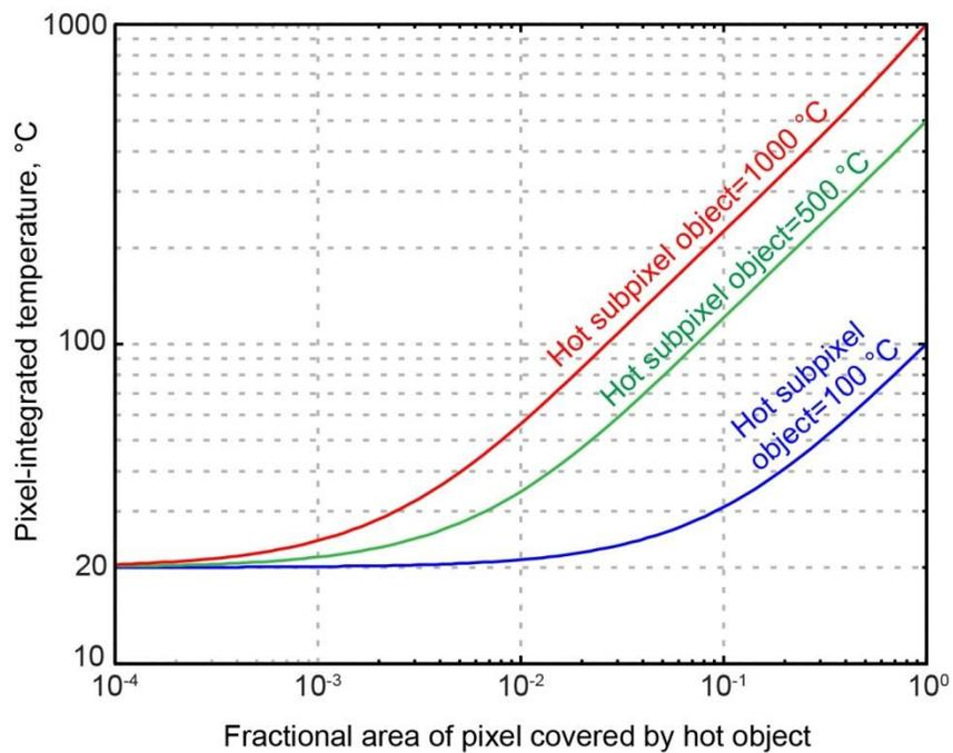
**Figure AF2-5.** Pixel-integrated temperature based on the fractional area of the pixel occupied by a hot object. Background temperature is assumed to be 20 °C.
