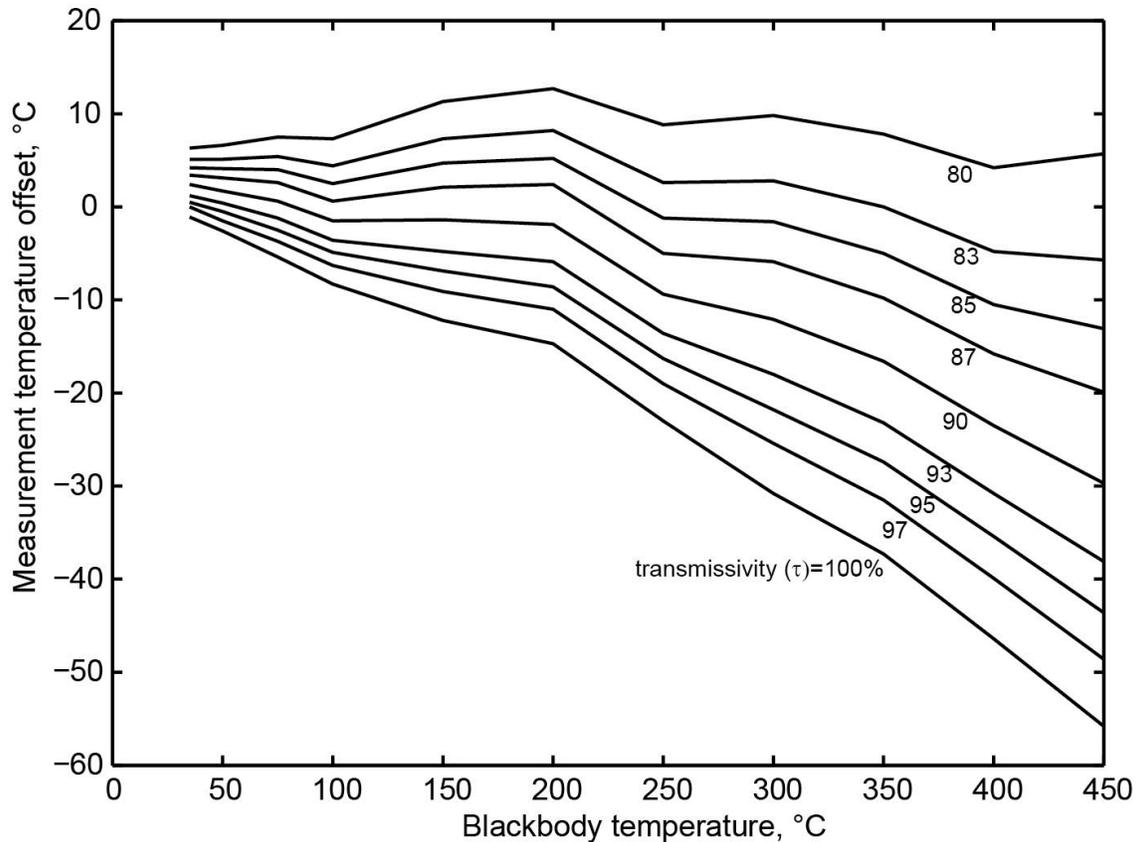
**Figure AF2-2.** Difference between measured and blackbody temperature for a range of transmissivity corrections for the ETcam looking through the germanium window (see Table AF2-1).
