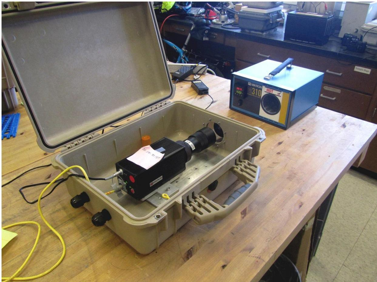
**Figure AF2-1.** View of calibration procedure using blackbody temperature source. The blackbody surface is inside the circular depression of the calibration unit. The camera is looking through the germanium window that is part of the enclosure.
